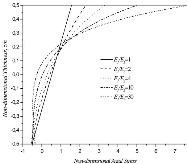
Fig. 7: Through the thickness distribution of non-dimensional axial stress  $\bar{\sigma}_x$  of the E-FG plate subjected to  $q = 1 \text{ KN/m}^2$  for different  $E_1/E_2=1$  in non-linear analysis.
