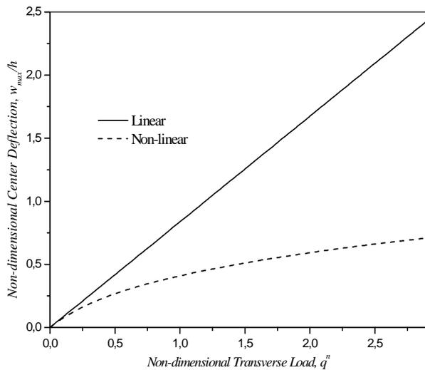
Fig. 2: Variation of the non-dimensional center deflection  $w_{max}$  of the E-FG plate versus  $q^n$ .
