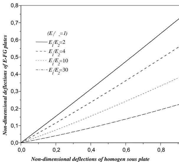
Fig. 8: Non-dimensional deflections of E-FG plates versus non-dimensional deflections of homogeneous plate for various material parameters in non-linear analysis ( $q = 1 \text{ KN/m}^2$ ).
