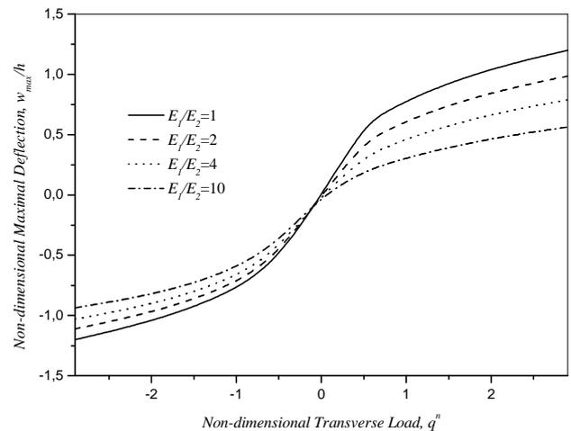
Fig. 5: Variation of the non-dimensional center deflection  $w_{max}$  of the E-FG plate versus  $q^n$  for different  $E_1/E_2$
