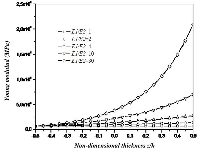
Fig. 1: The variation of the Young's module of an E-FG plate for different ratio of  $E_1/E_2$ .
