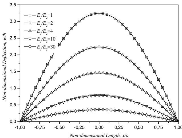
Fig. 4: Non-dimensional deflections due to transverse load  $q = 1 \text{ KN/m}^2$  versus non-dimensional length for different  $E_1/E_2$  in non-linear analysis.
